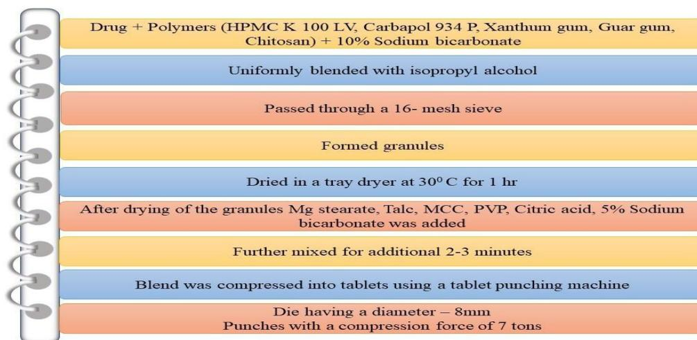
**Fig. 1: Direct compression method**
