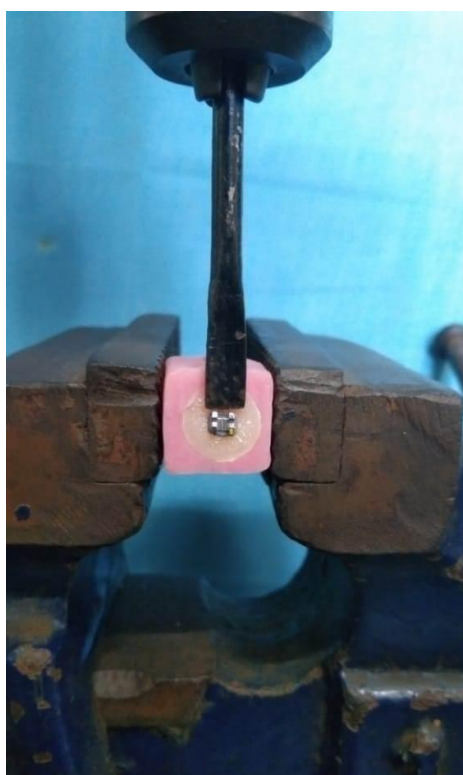
Fig 3 Shear bond strength testing
