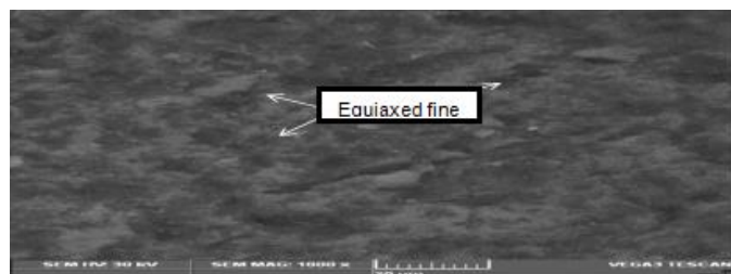
Fig. 11. c) SEM Image of welded region near AA2024
