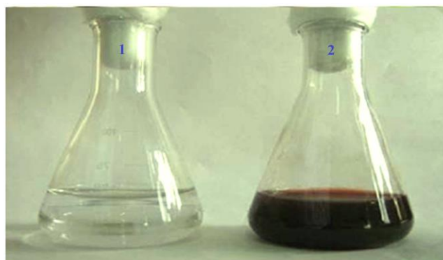
Figure 2. Color changes after the addition of leaf extract with aqueous silver nitrate solution: (A) silver nitrate solution (control), (B) silver nitrate with boiled leaf extracts
