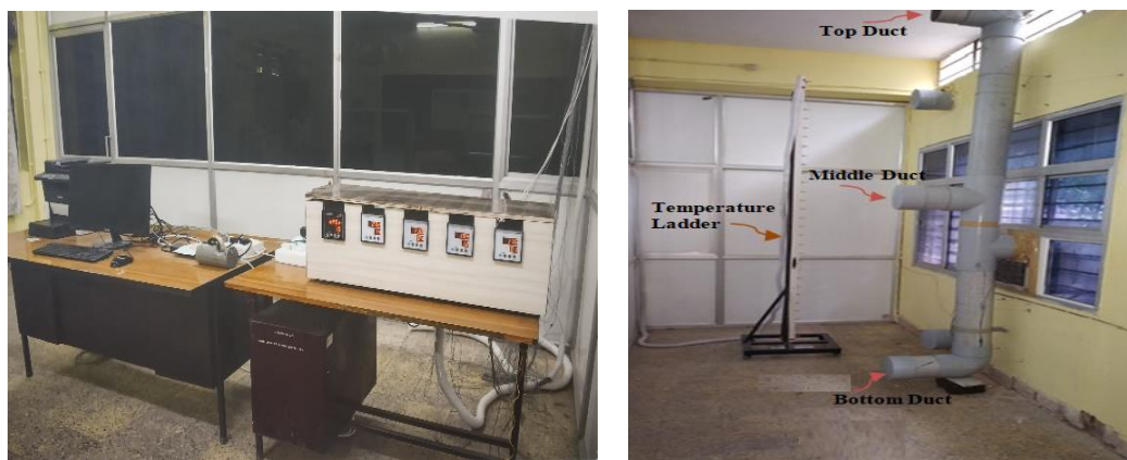
Figure 1: Experimental Setup a) Temperature Logger b) Test Room
