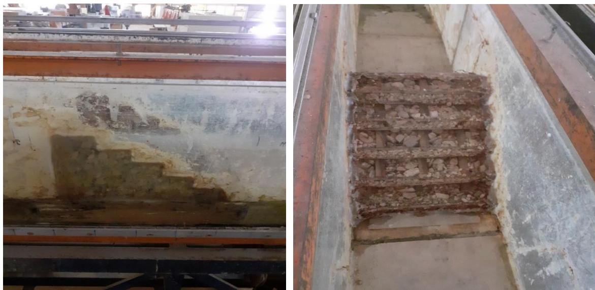
Figure (3) The experimental gabion stepped spillway model
