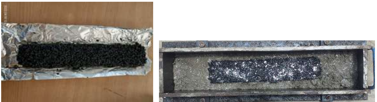
Fig. 1. (a) Cyanoacrylate Plate; (b) Cyanoacrylate Plate During the Casting
