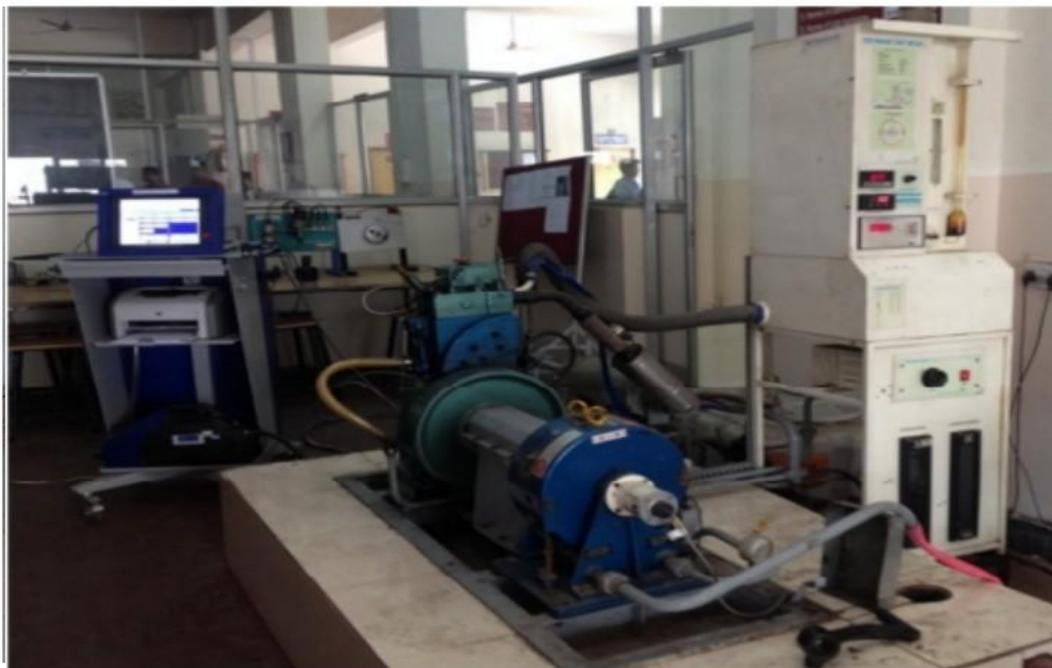
Figure 1 Test rig setup showing engine
