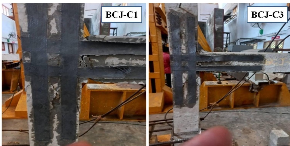
Figure 7(b) Crack patterns of 20% axially loaded CFRP retrofitted specimens
