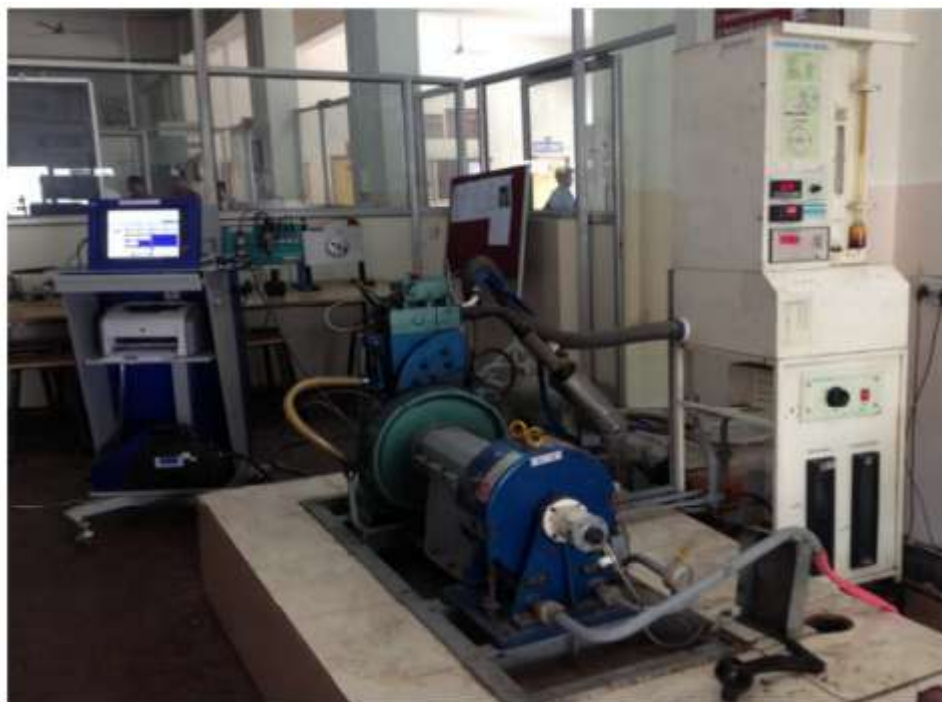
Figure 1 Experimental Setup with engine and analyzer
