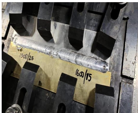
Figure 4 FSW (al to cu)
