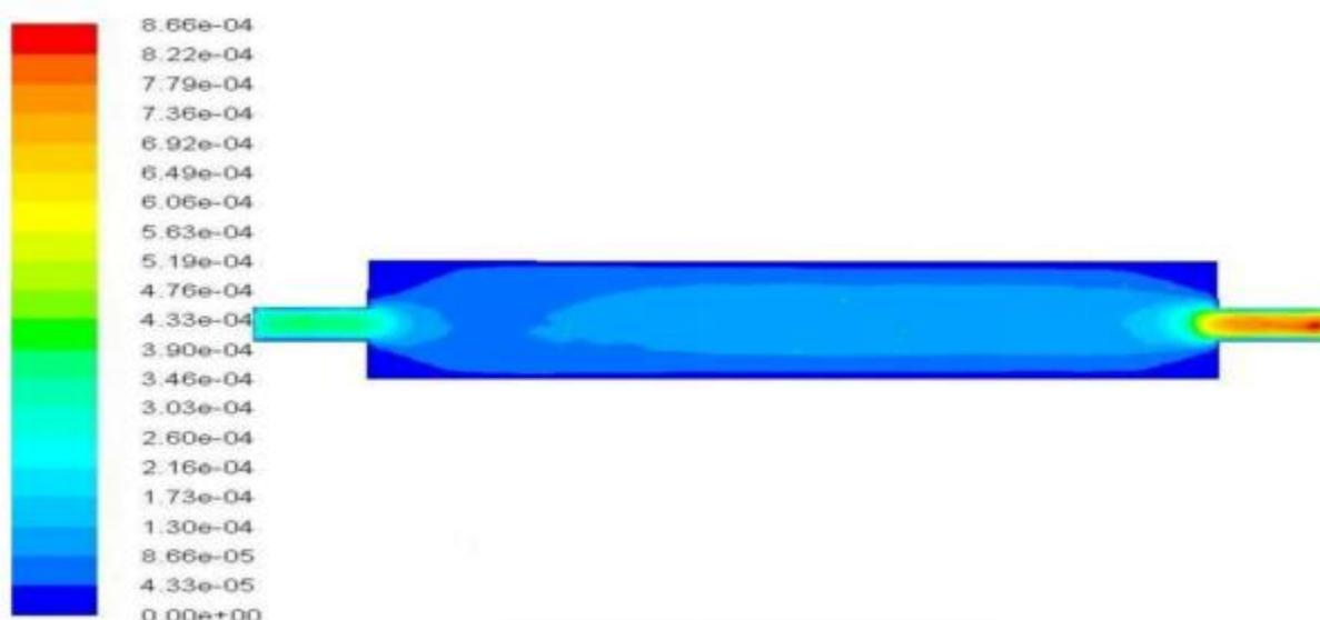
Figure No. 3 Distribution of velocity inside crystallizer at 400 seconds
