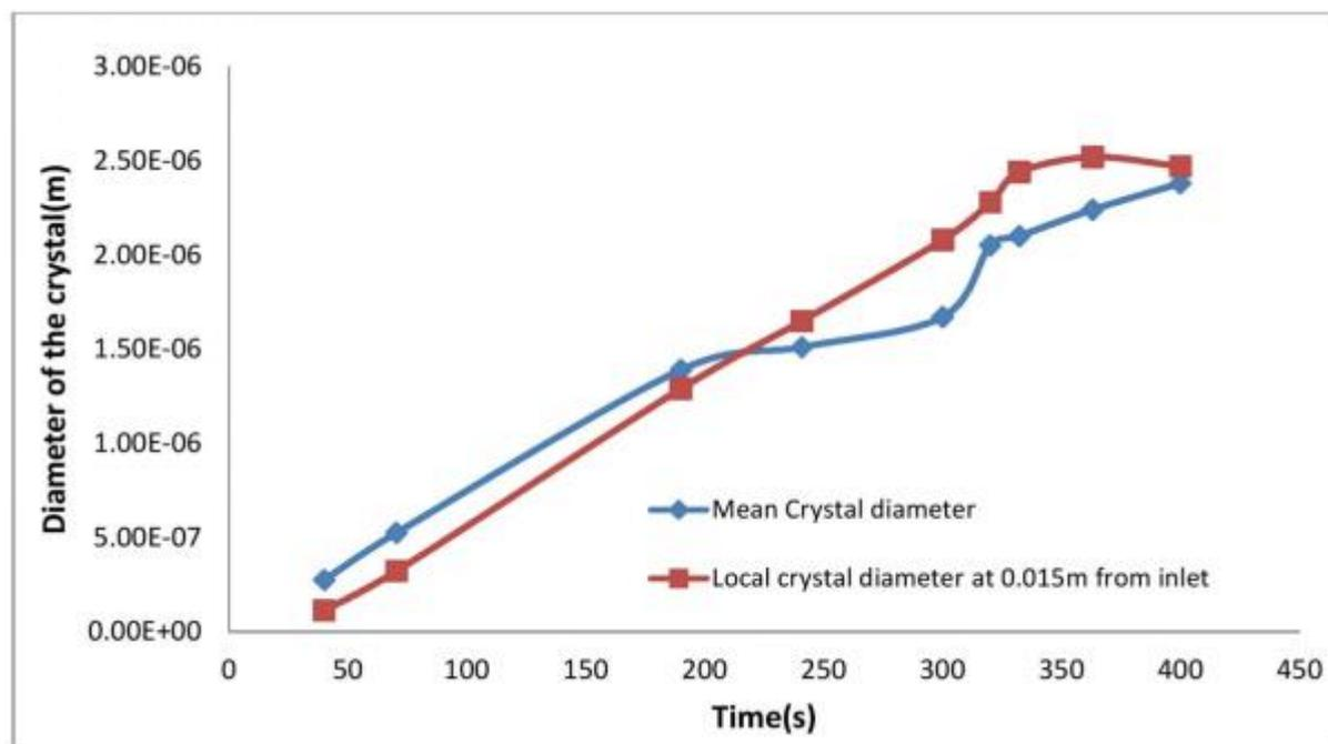
Figure No.1 Transient local crystal diameter distributions.
