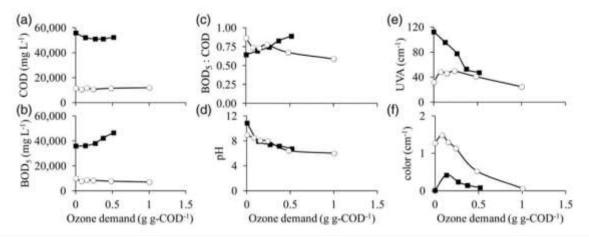
The graph displays the impact of ozone demand on the pharmaceutical company's strong stream (strong stream) (■) and bio-filter effluent (○) created in terms of (a) COD (b) BOD5 (c) ratio between BOD5 and COD, (d) pH, (e) UVA, (f) strong stream color.
