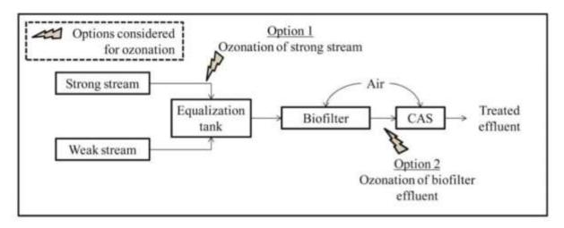
The pharmaceutical company's present wastewater treatment procedure is shown in the figure, along with the ozonation alternatives that were taken into consideration for this research.
