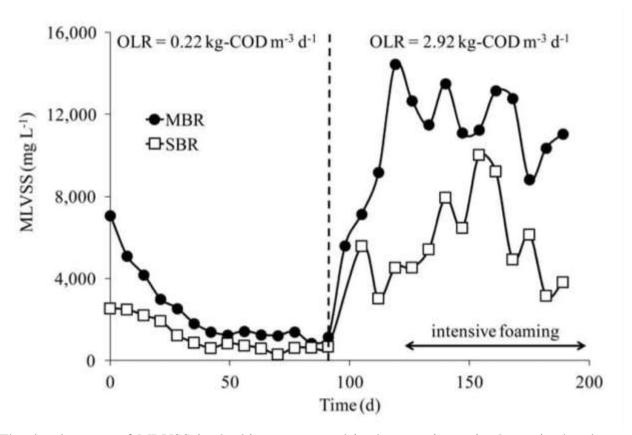
The development of MLVSS in the bioreactors used in the experiment is shown in the above figure with the OLR.
