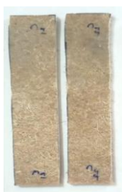
Figure 12 Tested specimen of Flexural Strength
