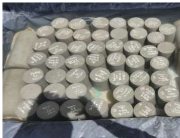
Figure 3. Cylinder curing well
