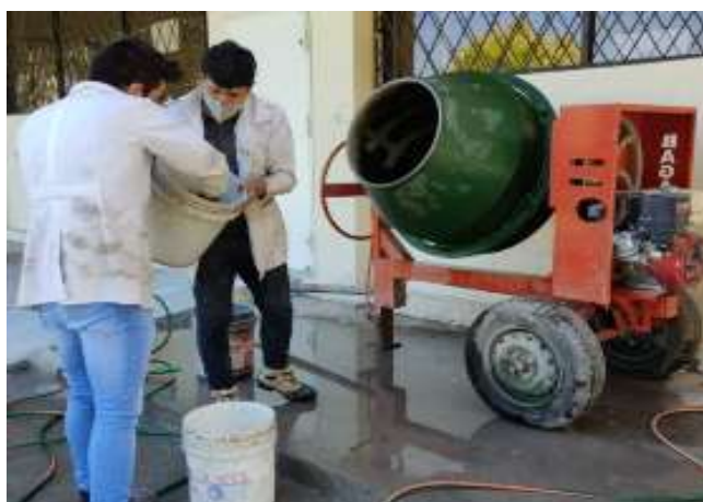
Figure 4. Adding water and superplasticizer to the mix
