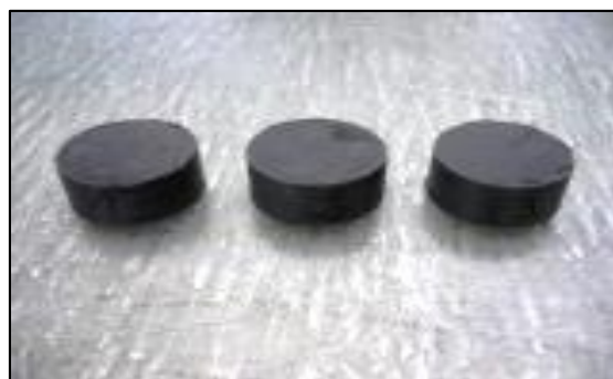
Figure 4. Photograph of Compression Set Specimen
