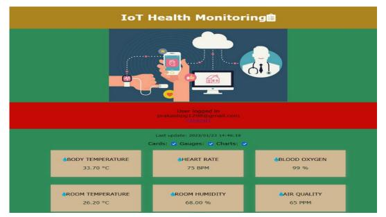
Figure 10. Displaying the real time sensed values in the created website
