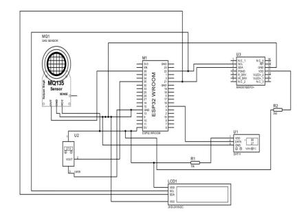
Figure 2. Circuit Diagram of our proposed IoT Health Monitoring System
