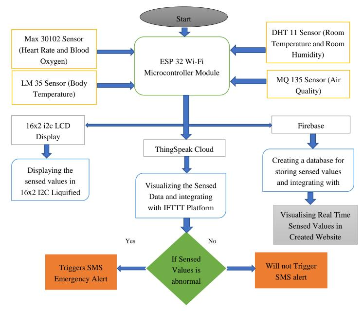
Figure 1. Flow chart of our proposed IoT Health Monitoring System
