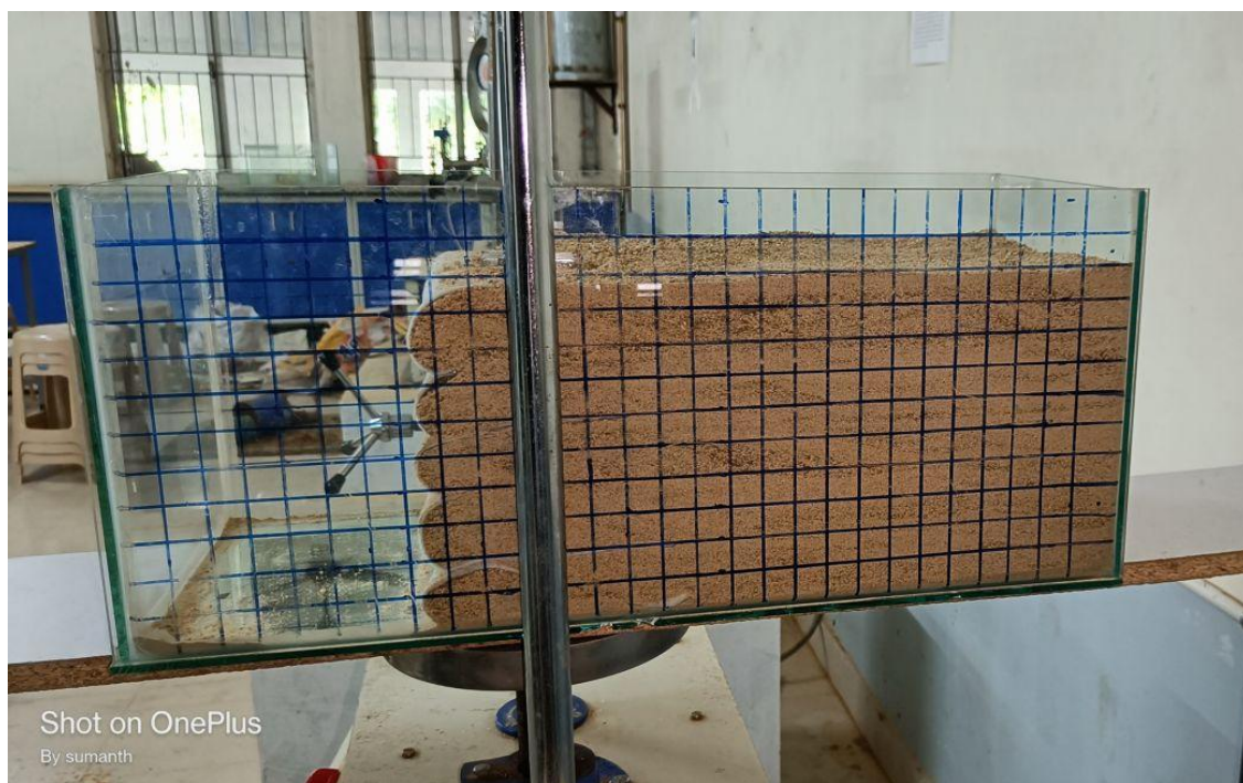
Fig. 2. Side elevation of the experimental set up of GRS retaining wall model
