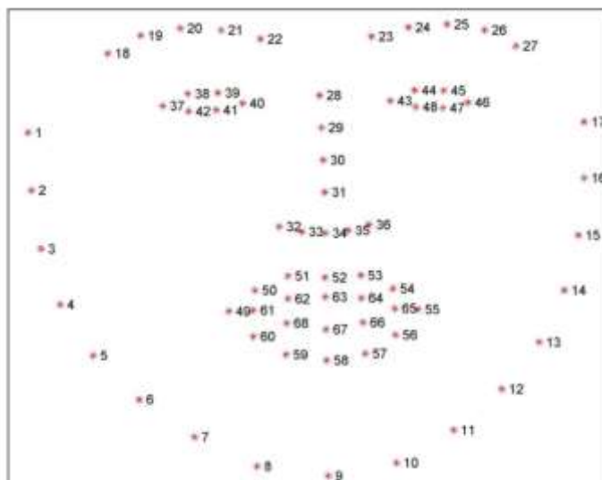
Fig. 1.The Dlib library provides a facial landmark detection feature that shows the location of 68 landmarks on the face. The SVM method divides these 68 elements into distinct sections such as left eye, proper eye, left eyebrow, proper eyebrow, mouth, nose, and jaw.
