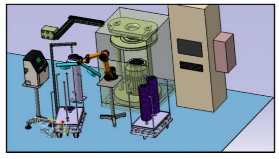
Figure 1 AUBO15 Robot with Electromagnetic Gripper in Clutch Diaphragm testing Process in DELMIA Software
