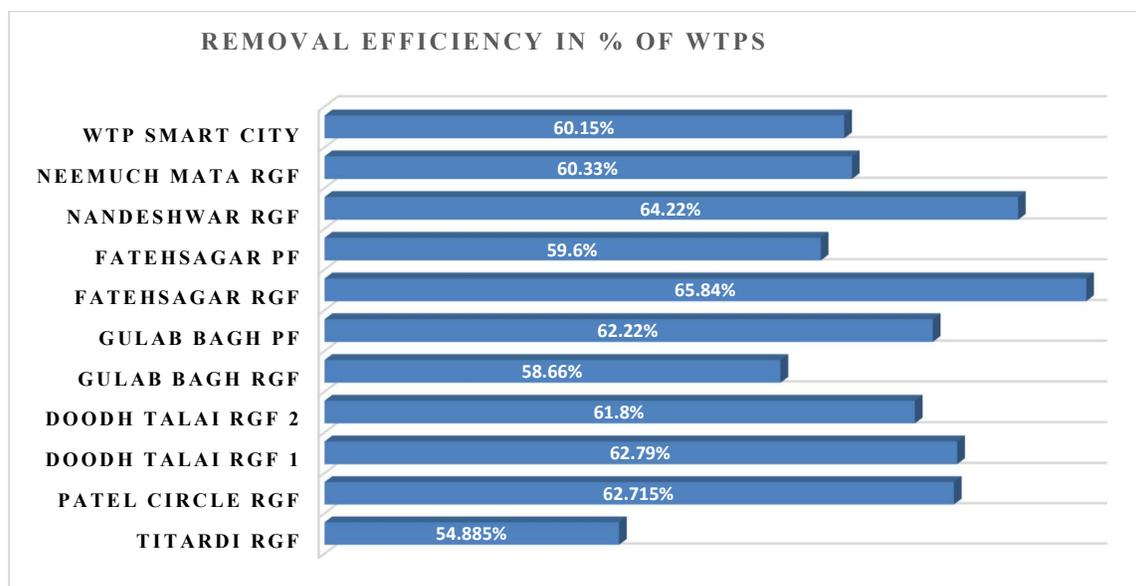
Graph 6: Comparison of Removal Efficiency in % of WTPS in Udaipur
