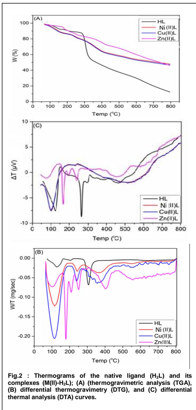
The DTA curves of the native ligand and its complexes (Fig. 2C) display weak and broad endothermic peaks at the temperature zone just prior to or accompanying the mass loss step in the corresponding TG thermograms.
