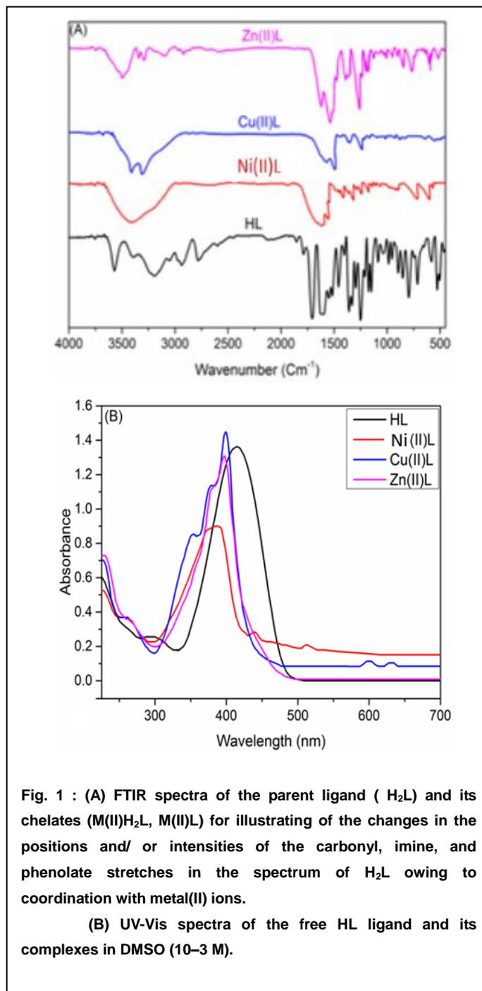
**Fig. 1 : (A) FTIR spectra of the parent ligand ( $\text{H}_2\text{L}$ ) and its chelates ( $\text{M(II)H}_2\text{L}$ ,  $\text{M(II)L}$ ) for illustrating of the changes in the positions and/ or intensities of the carbonyl, imine, and phenolate stretches in the spectrum of  $\text{H}_2\text{L}$  owing to coordination with metal(II) ions.**
