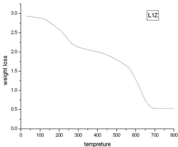
**Fig. 5 : Thermogravimetric analysis of Zn(II)H<sub>2</sub>L**
