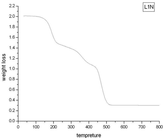
**Fig. 4 : Thermogravimetric analysis of Ni(II)H<sub>2</sub>L****TABLE 4**
