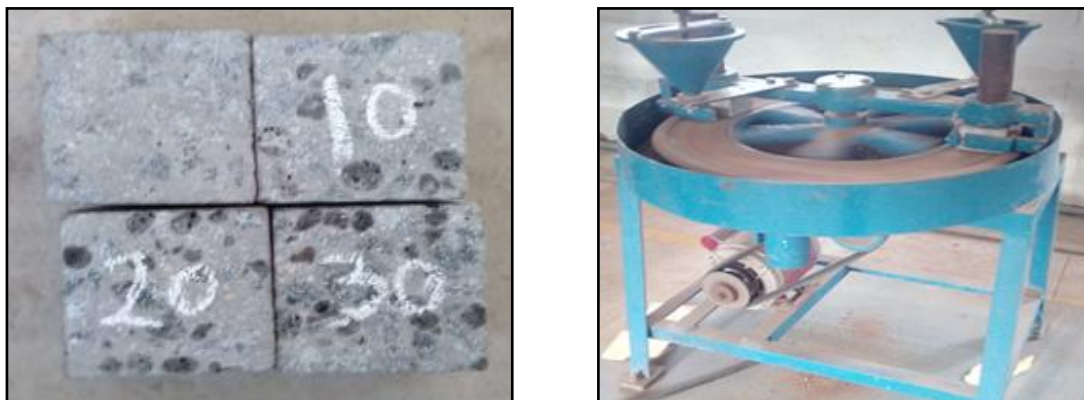
Fig. 11 Paver block Specimens for Abrasion test Fig.12 Abrasion test on paver blocks
