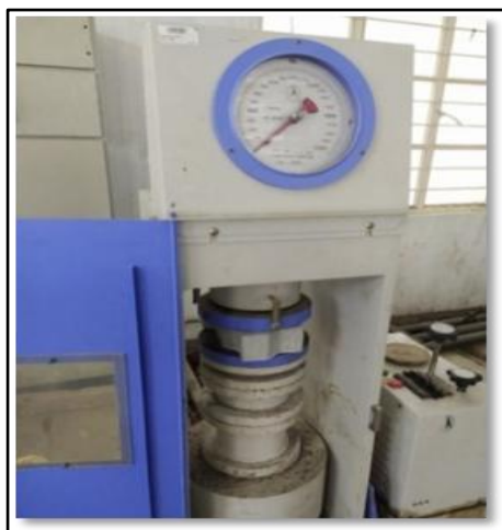
Fig. 4 Compression test on paver block specimen
