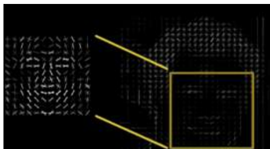
Figure.8 The HOG Image received by analyzing multiple images of the same Person.
