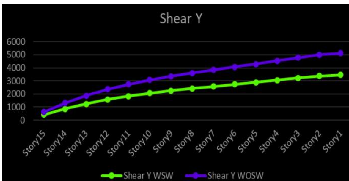
Figure 15: Storey Shear in Y Direction
