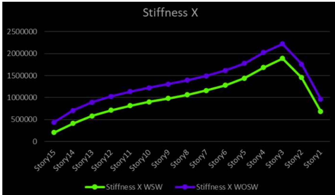
Figure 12: Storey Stiffness in X direction
