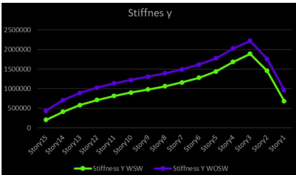
Figure 13: Storey Stiffness in Y Direction
