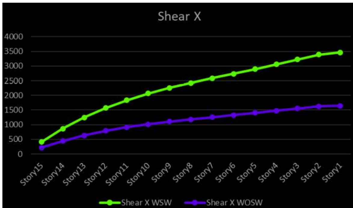
Figure 14: Storey Shear in X Direction
