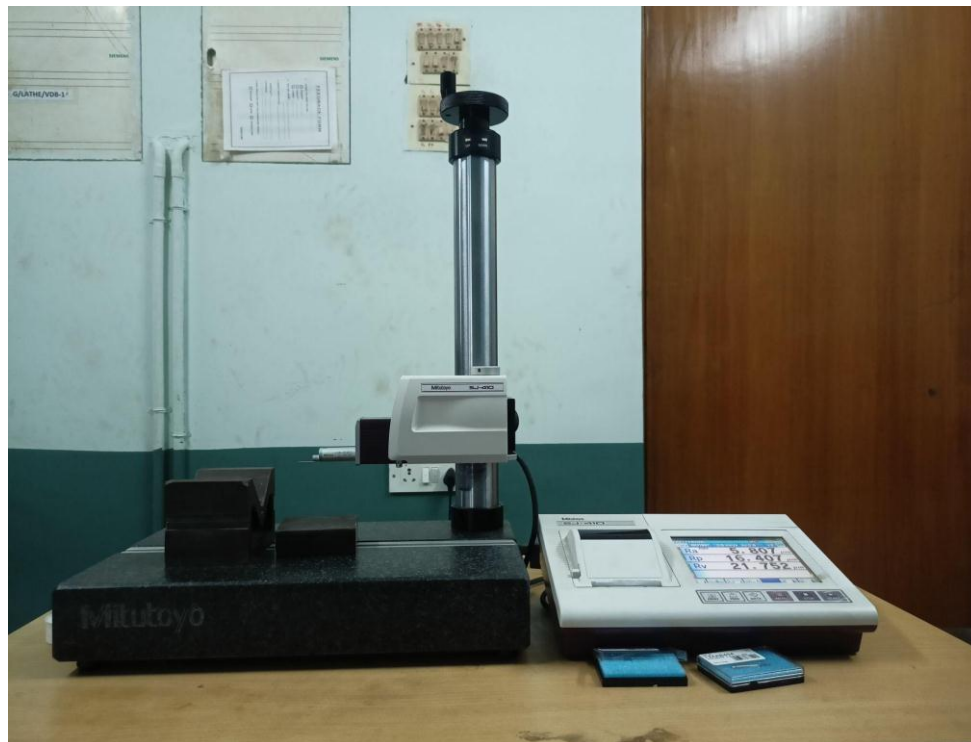
Fig. 5. Surface Roughness testing machine
