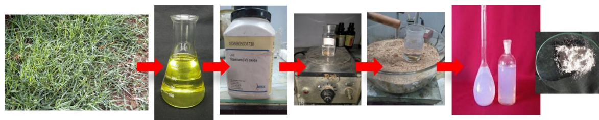
Scheme 1 Method for creating environmentally friendly TiO 2 nanoparticles by Cynodon dactylon (Doob grass)
