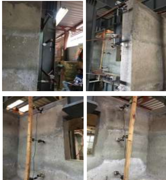
Fig.5 Arrangement of potentiometer and dial gauge
