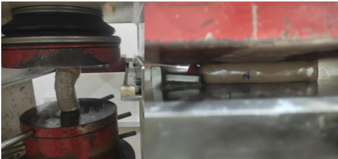
Fig 4: Failure mode a) PET brick in Vertical direction b) PET brick in a horizontal direction
