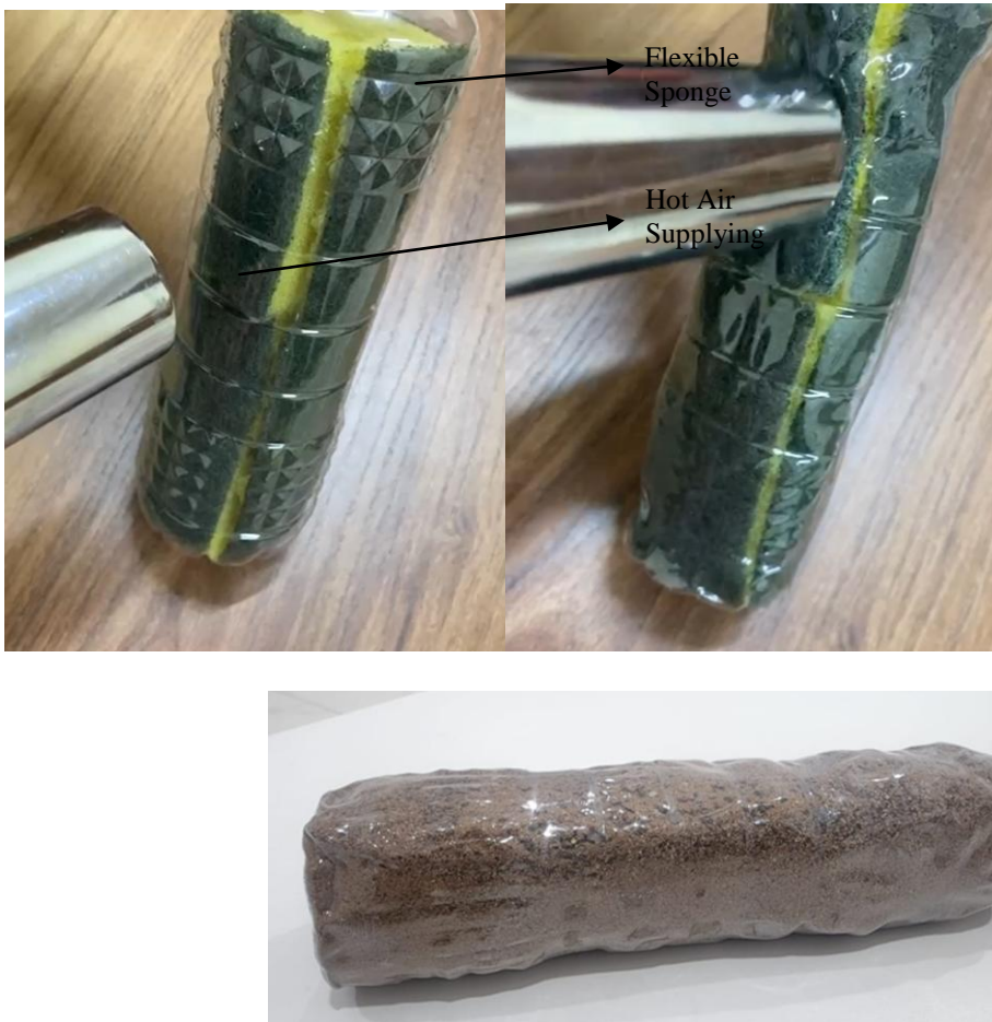
Fig 2: Experimental Process of preparation of PET Bottles (a) Before the application of Hot Air (b) During the application of Hot Air (c) PET bottle in quasi rectangular shape after sand/soil filling
