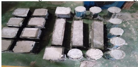
Figure 1 Cubes, Beams and Cylinder filled with SCC.
