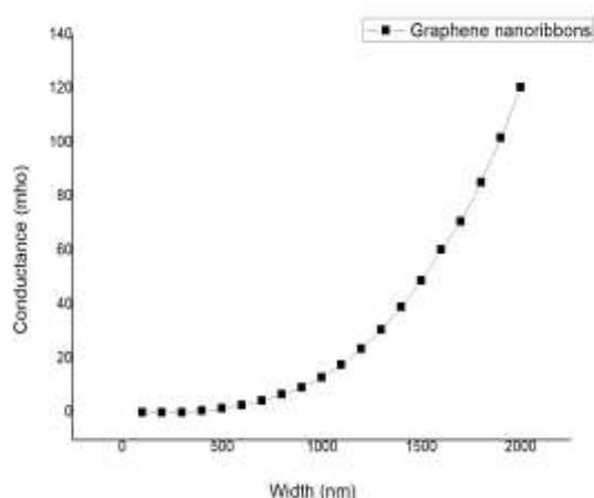
Fig. 2. Simulation of conductance of novel graphene nanoribbons with widths ranging from 50 nm to 2000 nm. The black line represents the conductance of graphene nanoribbons.
