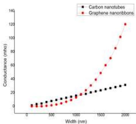
Fig. 3. comparison graph of conductance of carbon nanotubes and novel graphene nanoribbons. The Black line represents the carbon nanotubes and the Red line represents the graphene nanoribbons.
