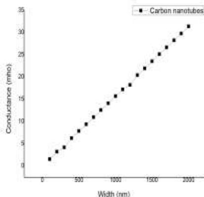
Fig. 1. Simulation of conductance of carbon nanotubes with widths ranging from 50 nm to 2000 nm. The black line represents the conductance of carbon nanotubes.
