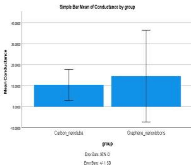
Fig. 4. Bar chart comparing the mean (+/- 1SD) conductance of carbon nanotubes and graphene nanoribbons. The mean conductance of novel graphene nanoribbons is better than carbon nanotubes. X-Axis: carbon nanotubes vs graphene nanoribbons. Y-Axis: Mean of conductance.
