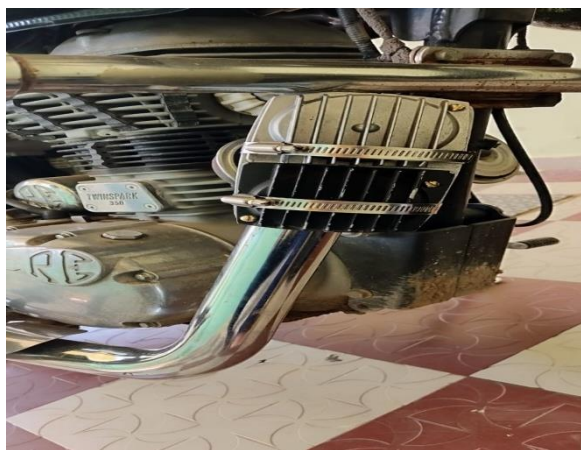
Fig. 2 Detailed shot of the silencer's installed Peltier module configuration.
