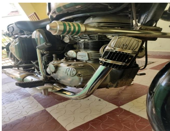
Fig.1.vehicle equipped with a Peltier module installed on the silencer
