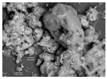
Coalesced or nano-clusters of nanoparticles (varied size of 86.5nm to 90.6nm)
