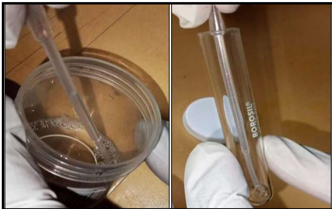
Fig 1.3: Saliva drawn into pipette and placed in test tube
