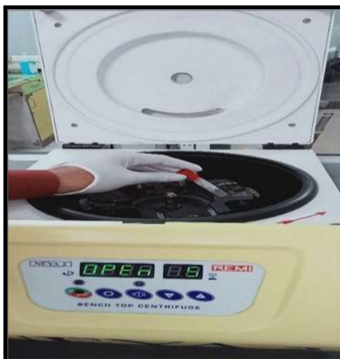
Fig 1.4: Saliva sample subjected to centrifugation at 3000 rpm for 15 minutes
