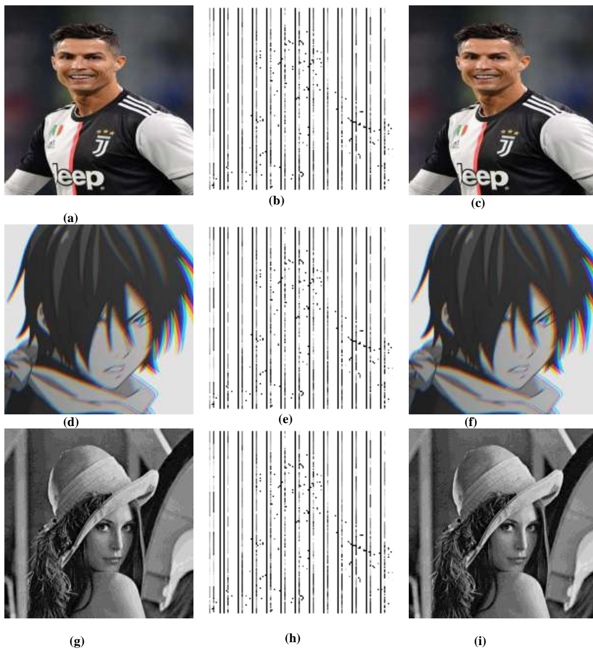
Fig. 2. DNA additive encoding Technique (a) sample image 1 ronaldo (b) encrypted ronaldo image using additive encoding (c) decrypted ronaldo image (d) sample image 2 anime (e) encrypted anime image using additive encoding (f) decrypted anime image (g) sample image 3 lenna (h) encrypted lenna image using additive encoding (i) decrypted lenna image.
