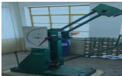
Figure 3 Izod impact testing machine used for evaluating the impact strength. Capacity: 300 J, Overall size: 1.4 x 0.5 x 1.9, Net weight: 450 Kgs
