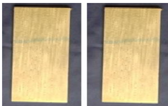
Figure 1 Aluminium foam core with different thickness (0.5 & 1 mm) sandwiched with glass fibre epoxy laminate
