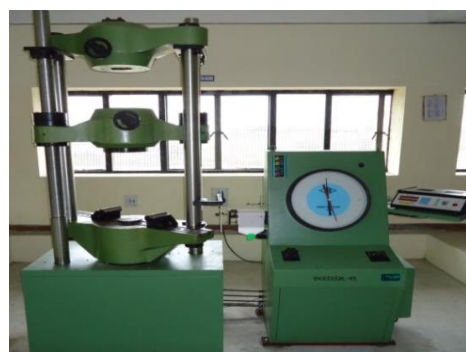
Figure 2 UTM machine used for evaluating the tensile strength. Capacity: 10 KN, Maximum cross head travel: 1100 mm, Testing speed range: 0.001 to 1000 mm/min, weight: 115 kg
