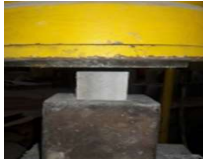
Fig2. typical test setup for compressive strength [16]
