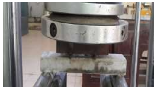
Fig 3.flexural strength testing set-up [16]
