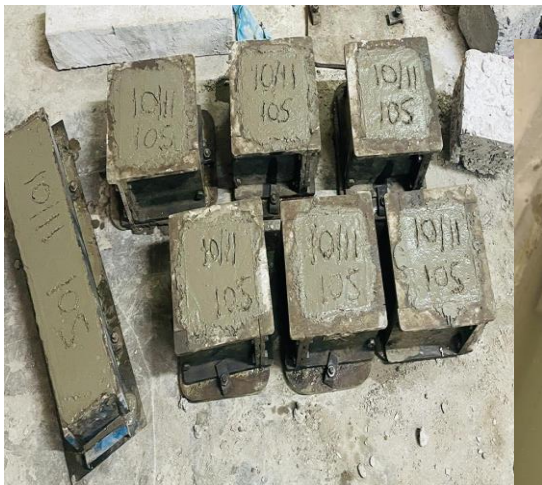
Fig 3: Casted cubes and beams
