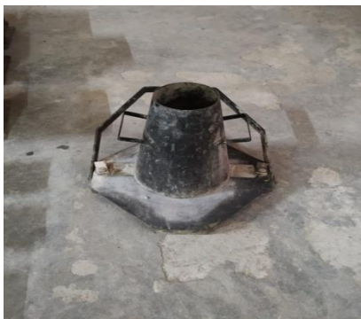
Fig 1: Slump Cone Apparatus
