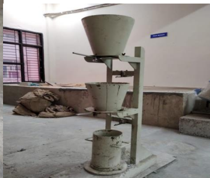
Fig 2: Compacting Factor Apparatus
