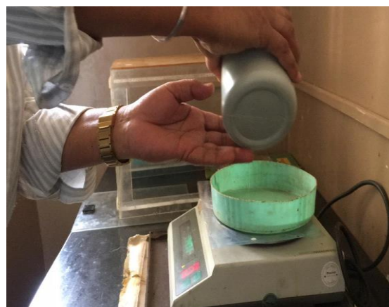
Figure2. Mixing of Polyester resin with Catalyst and accelerator
