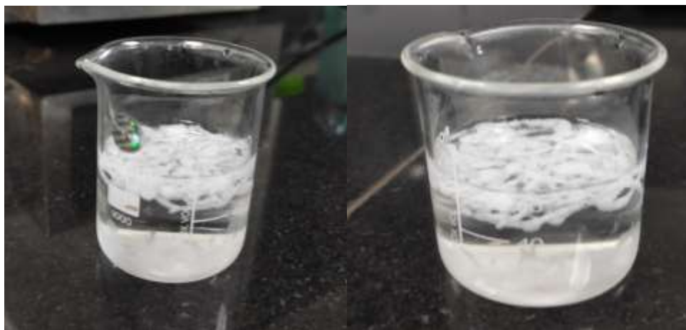
Figure 5: Photograph of floating and gelling behaviour of in-situ gel
