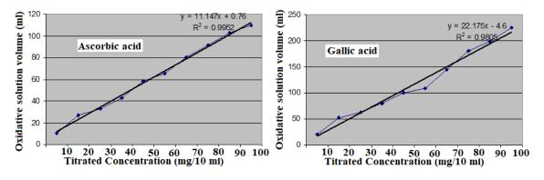
Figure 4. Calibration curves of oxidative titration of ascorbic/gallic acid with permanganate.
