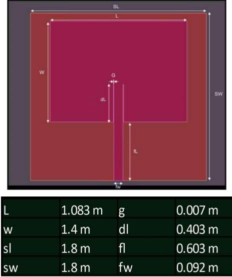
Figure 1: The patch antenna structure
