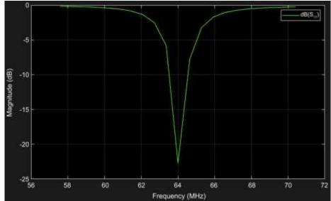
Figure 2: S11 parameter exhibiting 20 dbs magnitude radiation at 64 MHZ
