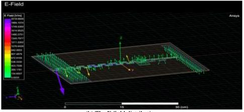
(b) The E field distribution Figure 7: Future suggested antenna, (a) antenna construction, and (b) field dispersion for wearable device
