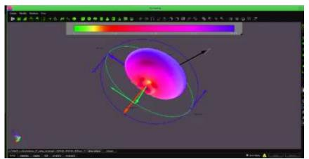
Figure 4: The distribution of the E field from the feed area at x = 0 to Emax at 8.5 V/m
