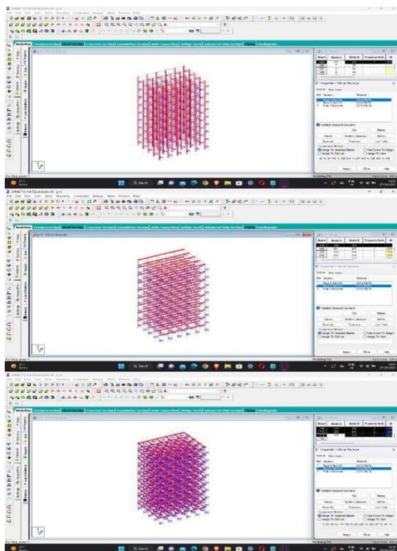
to be 2.25KN/m. Following the guidelines of IS1893:2002, the seismic load was applied to the building in both the X and Z axes.
