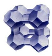
Fig 4. Molecular Sieve Type A
