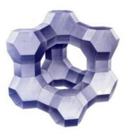
Fig 5. Molecular Sieve Type X
