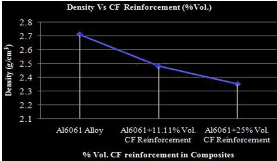
Figure 9: shows the density of composites using CF reinforcement and aluminium 6061 alloy
