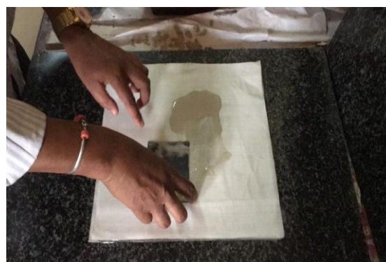
Figure3. Hand Layup Process
