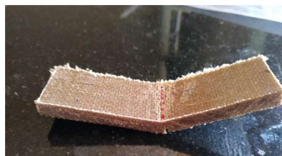
Figure6. Flexural test after failure
