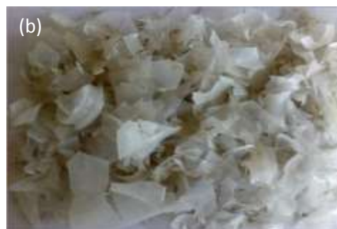
Figure 1. (a)Raw material from Clinical Lab waste as a Glucose bottle (b) Shredded sample of the Glucose bottle after process
