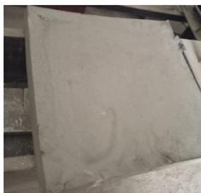
Fig 7: Non-porous geopolymers slab
