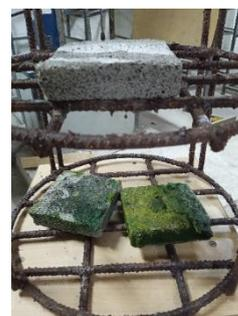
Fig 16. Experimental setup Fig 17a: Before carbonation Fig 17b:After carbonation
