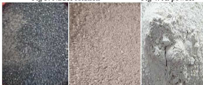
Fig 5: Dry mix materials (Copper Slag , Fly ash , GGBS)
