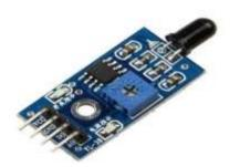
sources. In general, this sensor picks up IR (Infrared) light with a wavelength of 760 nm to 1100 nm that is released by the fire flame or other light source.
