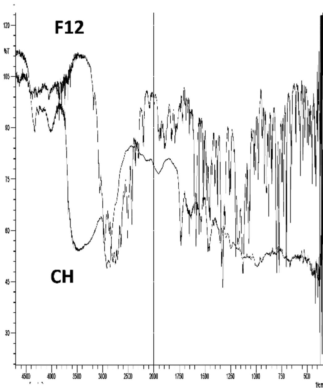
Fig. 3: FT-IR study for pure drug powder CH and selected liquisolid formulation (F12)
